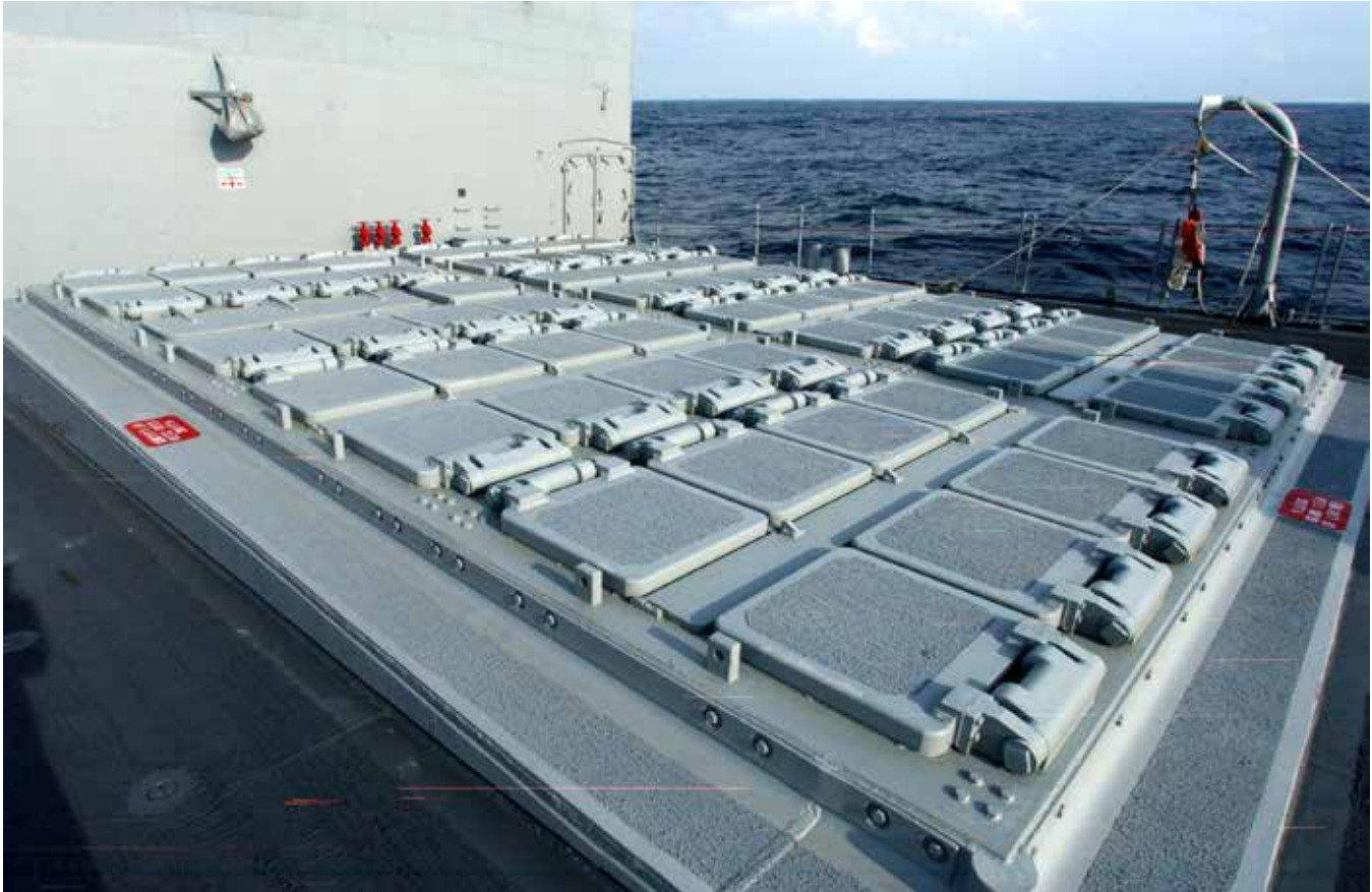
The multi-purpose launch tubes of the MK-41 Vertical Launching System (VLS).
