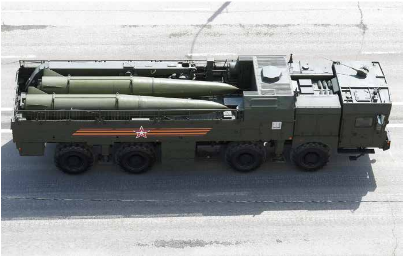
Iskander-M short-range missile was designed to penetrate air and missile defense systems.
